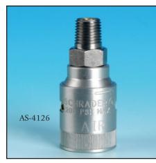
Schrader Medical twist-release gas connectors are safety-keyed for air. This quick connector safely handle up to 200 psi. Design prevents interchangeability of major internal parts for different gases. They are UL certified and comply to NFPA 99 (2002 edition).
